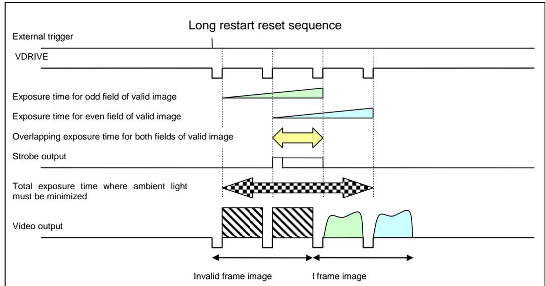
The camera is configured for frame accumulation mode, the electronic shutter is disabled and the restart reset mode is enabled. The camera receives a permanent HDRIVE horizontal synchronization signal from the frame grabber.
