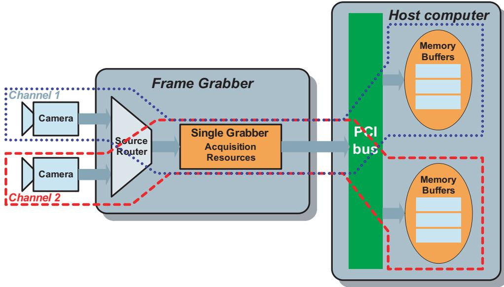
The source router on the figure operates as a switch and allows MultiCam to select one of the two cameras.
