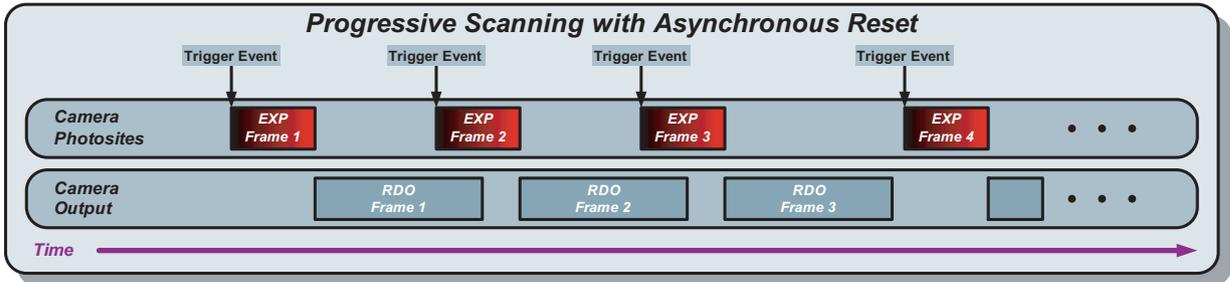
A trigger event external to the camera marks the beginning of the exposure period. When the camera is able to start an exposure period before the end of the previous readout period, an expose overlap occurs. This mode of operation offers the highest frame rate achievable.
