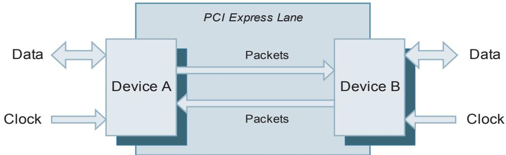
The delivery bandwidth from and to a device is increased by using multiple lanes in parallel. The PCI Express architecture permits the parallelization of 1, 2, 4, 8, 12, 16 and 32 lanes. This parallelization only involves the hardware layer and is application transparent.
