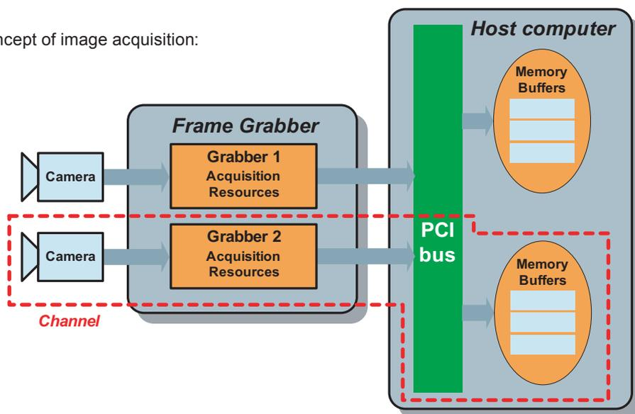
MultiCam allows control of the full acquisition path between the camera and the host computer memory with a MultiCam object called **channel**. The channel is under the control of the user application. The channel represents what is surrounded by dotted lines on the above picture. All components of the channel are examined below: the camera, the grabber and the memory buffers.
