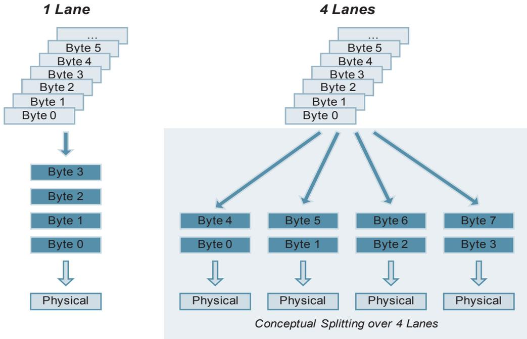
The theoretical usable data rate of one PCI Express lane reaches about 200 MByte/s in each direction (for a total of 2 x 200 MBytes/s).
