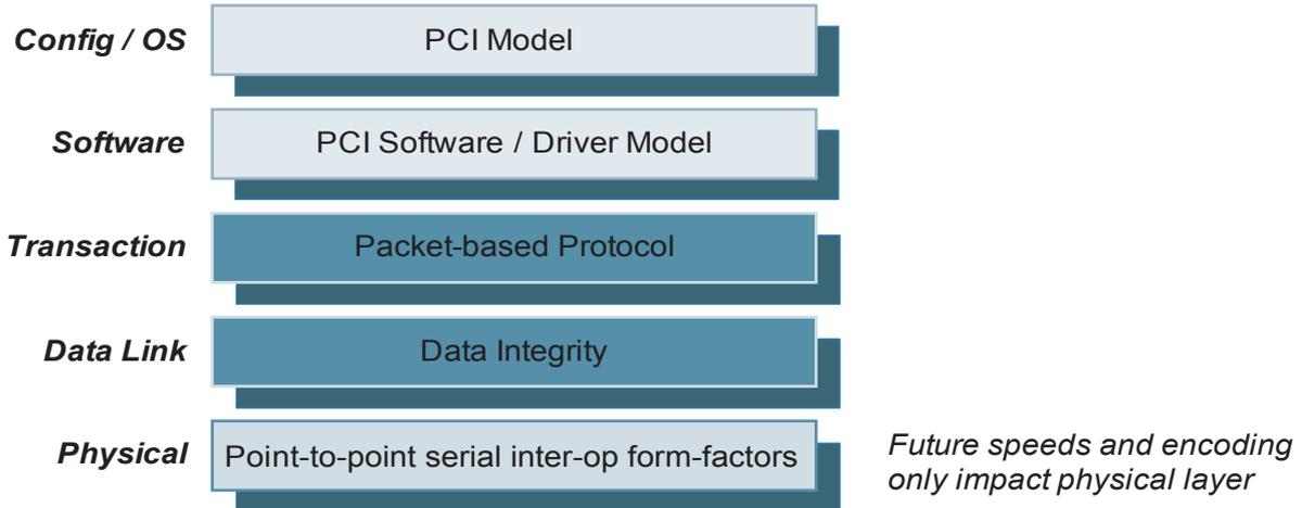
PCI Express software layers are backward compatible with Conventional PCI. Applications moving from Conventional PCI to PCI Express architecture do not require software upgrading.
